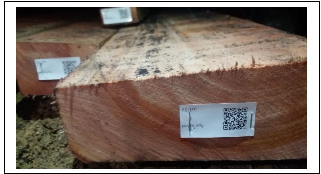
Printed lumber labels are stuck at the end of each lumber
