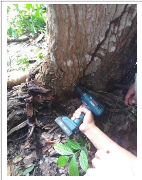
Fig. 4. Drilling a guide hole and hammering an RFID nail tag during timber inventory.
