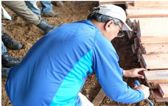
QR code labels attached to end of each lumber is secured with staple wire.
