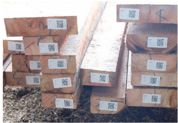
QR code labels attached to end of each lumber is secured with staple wire.
