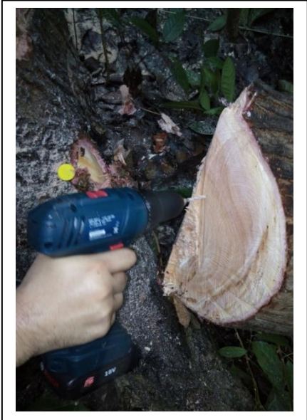
Drilling Guide Hole on one Log End
