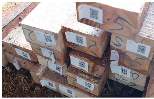
Log RFIDs and lumbers produced with the assigned log number label using lumber crayon
