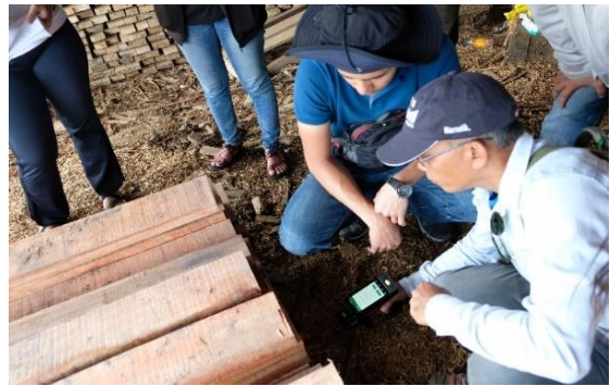
Scanning and association of log RFID with the lumber labels. And request for transport document (Certificate of Lumber Origin-CLO).
