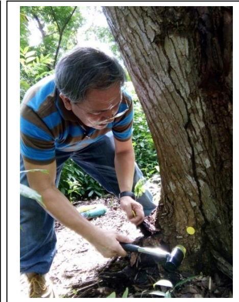
Fig. 4. Drilling a guide hole and hammering an RFID nail tag during timber inventory.
