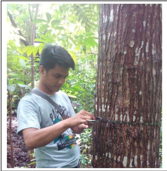
Fig. 3. Measuring Tree Diameter using diameter tape and Merchantable and Total Tree Height using Laser Range Finder.
