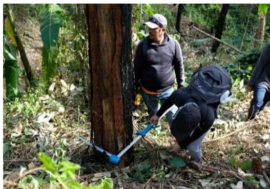
Diameter measurement using a Tree Caliper, drilling guide holes, implanting RFID Nail Tags and encoding of the trees inventoried in the Handheld Device.
