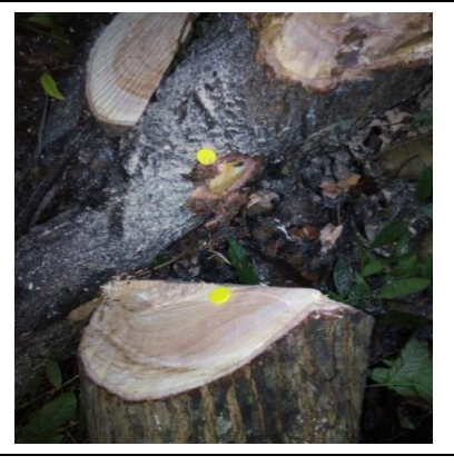
RFIDs Inserted on a Tree Stump and the Log Derived from the Tree Stump
