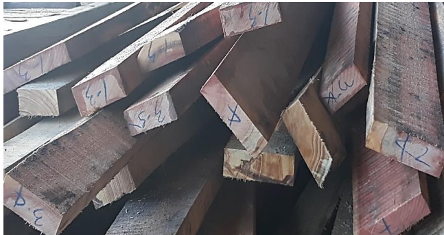
Log RFIDs and lumbers produced with the assigned log number label using lumber crayon
